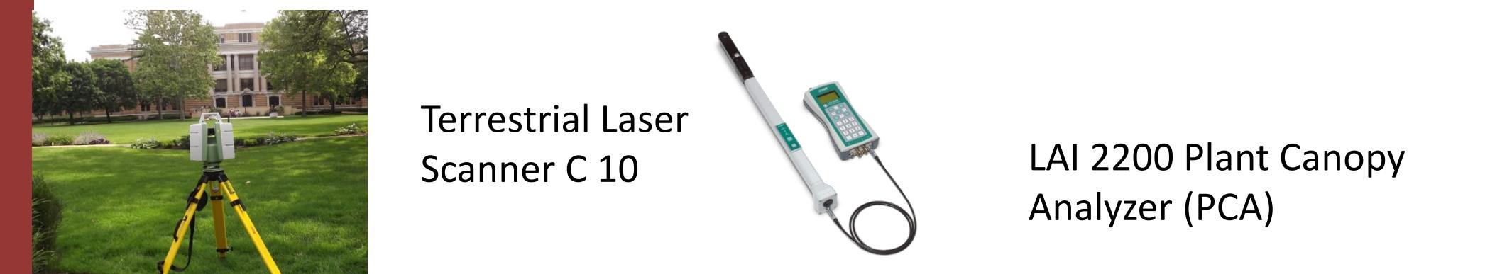
At each site, 4 scans were acquired and co-registered into a single point cloud. The co-registered point clouds were clipped to a 30 m radii surface area. PCA data were collected from 9 positions from each site.
