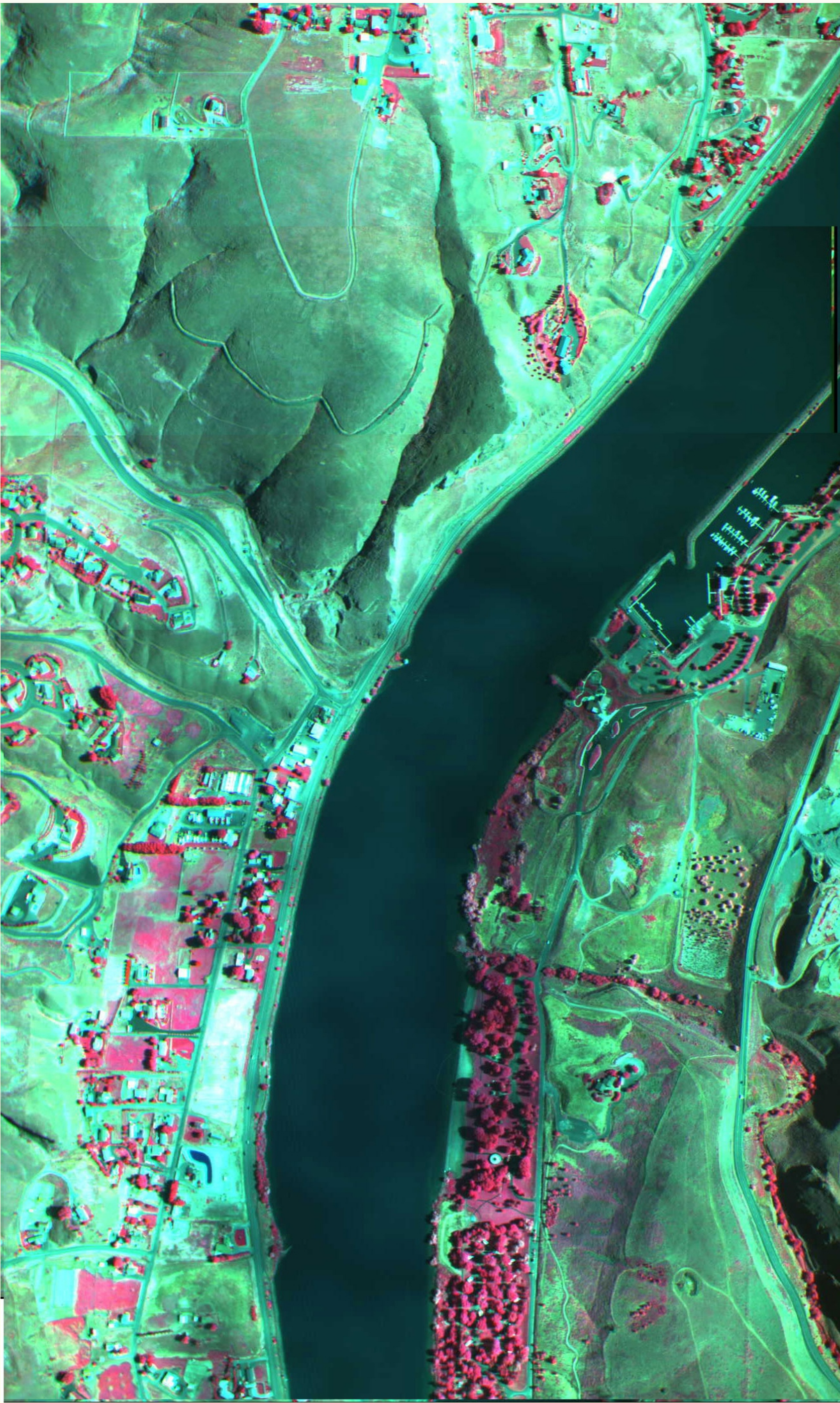
True and false color imagery of Hells Gate State Park, Lewiston ID (acquired June 2005 with HAMCAM's multispectral imager at 7000 ft AGL)
